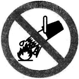
Do not extinguish with water
